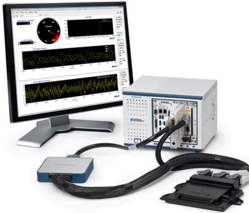
**Figure 4. A typical hardware and software combination for an electric motor ECU HIL test**
