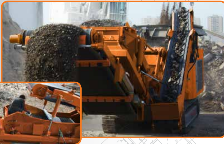
Maintenance timesaving due to hydraulic cylinders on the screenbox.
