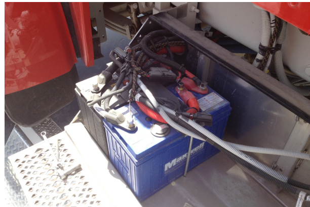
The Maxwell Engine Start Module installed with three lead-acid batteries in a Class 8 tractor (left) and in a day cab ready-mix truck with one battery (right).
