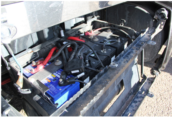
The Maxwell Engine Start Module installed with three lead-acid batteries in a Class 8 tractor (left) and in a day cab ready-mix truck with one battery (right).
