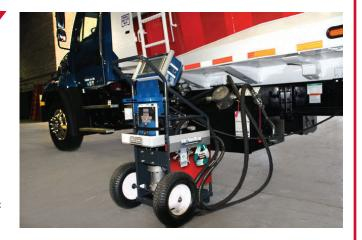
Working closely with the supplier as well as the refuse haulers, Schroeder created a way to monitor, filter (and most importantly) record this critical information. The Asset Management Filtration Station® provided all of this in one, mobile filter cart. The built-in computer and custom software provides complete visibility to service managers on the status and routine maintenance of the vehicle.
