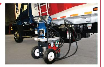
Working closely with the supplier as well as the refuse haulers, Schroeder created a way to monitor, filter (and most importantly) record this critical information. The Asset Management Filtration Station® provided all of this in one, mobile filter cart. The built-in computer and custom software provides complete visibility to service managers on the status and routine maintenance of the vehicle.
