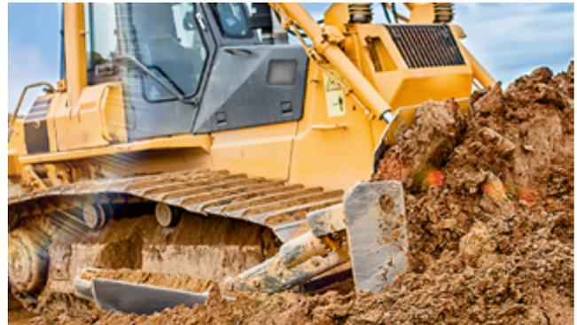
in parallel with ground speed requirements to optimize vehicle performance. Using a combination of motors, speed sensors, pressure transfers and built-in software intelligence, it is possible to dynamically readjust how much power is sent to each side of the machine — providing better control over vehicle direction, movement and speed.
